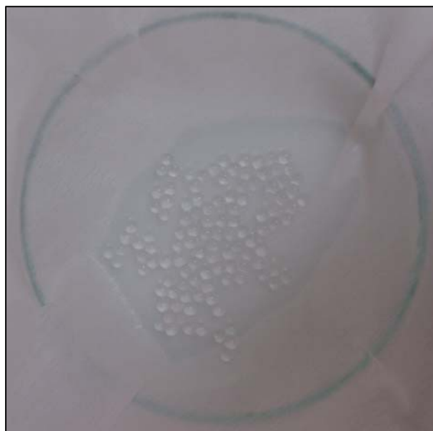
Figure 1. Alginate beads produced by 2% alginate and 50 mM Ca 2+
