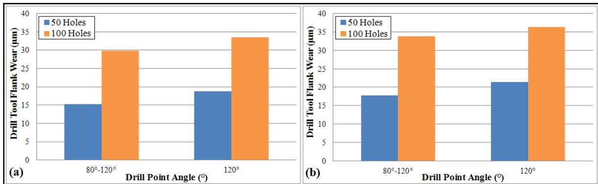
**Figure 5.** Drill tool flank wear according to the drill point angle ( $V=40$  m/min,  $f=0,1$  mm/rev), a) HDPE and b) CBR-HDPE.
