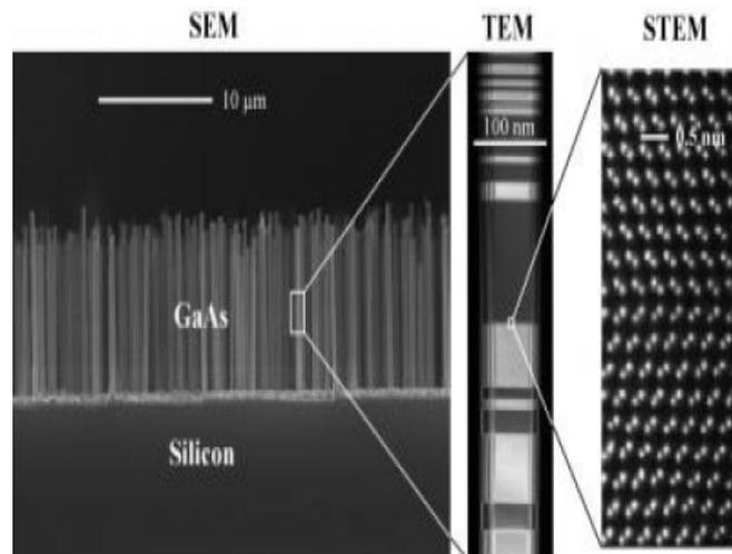
**Figure 5.** Schematic structure of the nanowires naturally concentrate the sun's rays into a very small area
