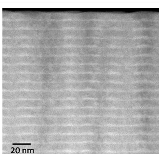
**Figure 3.** TEM image of self-organized quantum dot superlattice
