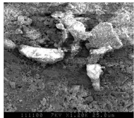
Figure 5: Cross section SEM micrograph on sandblasted steel (Sa2.5).
