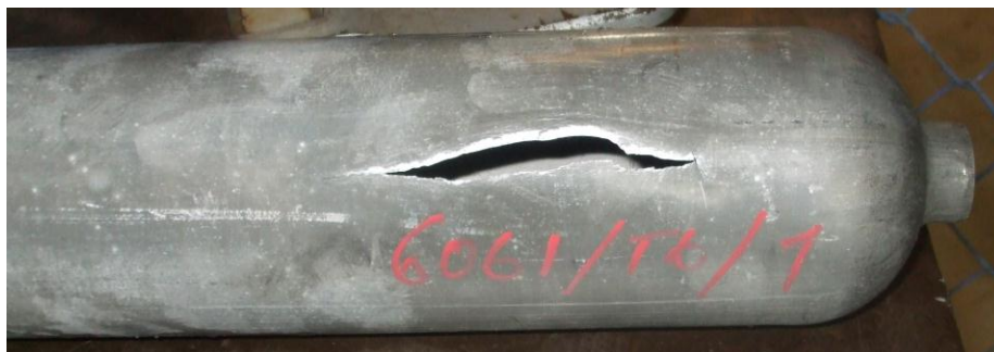
Figure 10. View of 6061 T6/1 Sample After Hydrostatic Pressure Test
