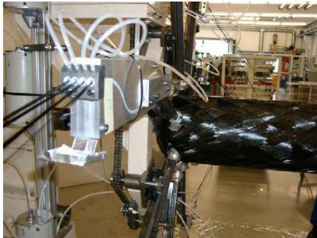
Figure 1. Wrapping of Carbon Fiber Supplementation on the Aluminum Tank (Rau and Colom, 2006) Since the beginning of 2000, works have been done on the usage of hydrogen in vehicles. In this context, many prototypes are produced and after completion of tests vehicles brought in use. In many countries, there are hydrogen refueling stations.
