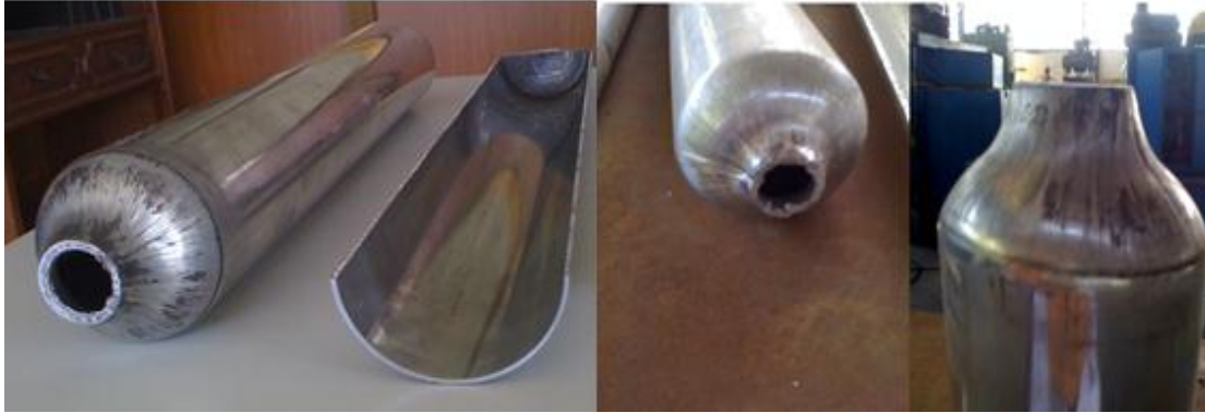
Figure 5. Shrinking process for end part of the Aluminum-hydrogen tank
