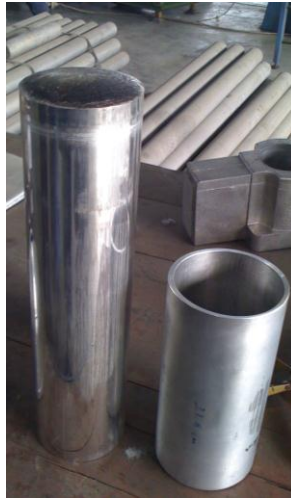
Figure 4. The comparison between first forming process and second forming process
