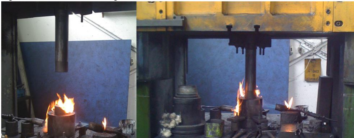
Figure 2. Getting a hollow cylinder shaped as a container from a filled cylinder by the help of a press With the pressure of male mold, the material in the female mold is plastered on the male mold. In the first stage with the help of press a draft hollow cylinder is obtained from full material. In the next stage the length of the tank will be extended by reducing the wall thickness with height extension process as shown in Figure 3.
