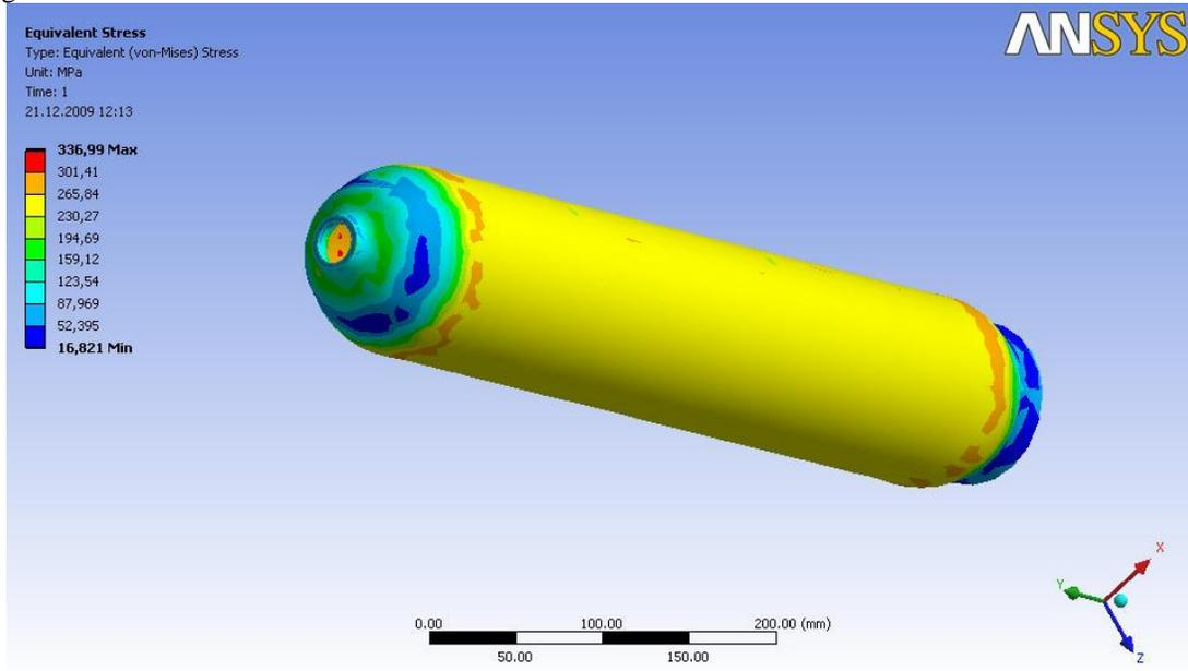
Figure 9. 6082 T6 201 Bar ANSYS Equivalent Stress Results
