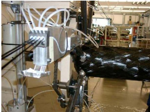
Figure 1. Wrapping of Carbon Fiber Supplementation on the Aluminum Tank (Rau and Colom, 2006)
