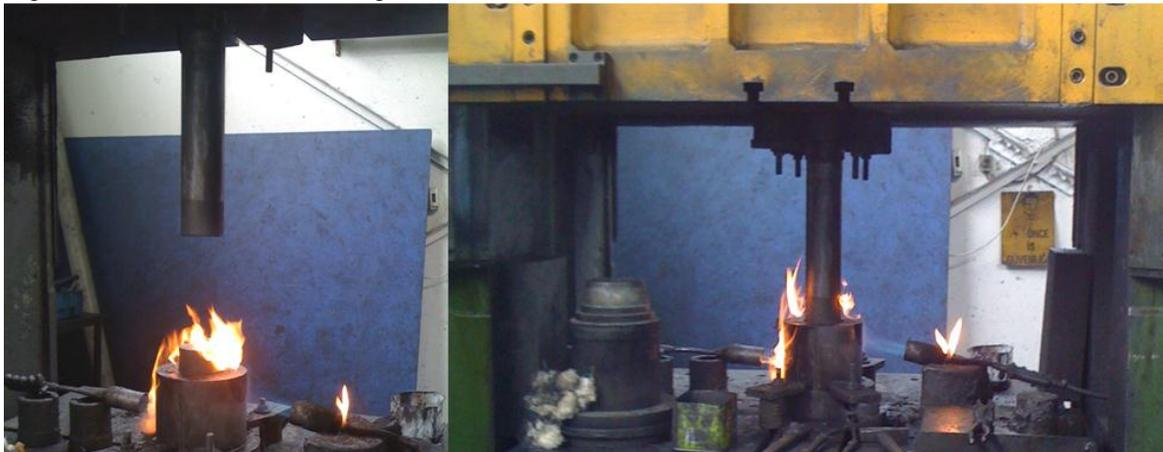
Figure 2. Getting a hollow cylinder shaped as a container from a filled cylinder by the help of a press
