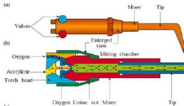
Fig. 5: Oxyacetylene Welding
